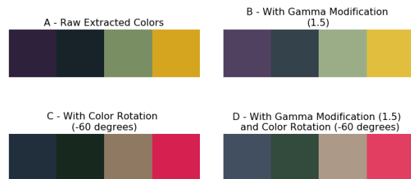
Fig. 3. (A) The colors extracted from the four panels of a pH strip, stored in code as a total of 12 RGB values. (B) Gamma correction with a parameter of 1.5 applied on the raw extracted colors. Gamma correction nonlinear maps each color to effectively lighten or darken the image. (C) Hue rotation of -60 degrees around the color wheel applied on the raw extracted colors. (D) Application of both a gamma correction of 1.5 and a hue rotation of -60 degrees on the raw extracted colors.
